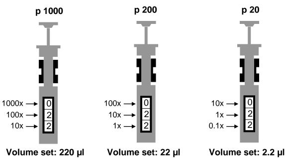
In a P100, the top number refers to 1000's of µl, the middle number refers to 100'sµl and the bottom number refers to 10's of µl's.
