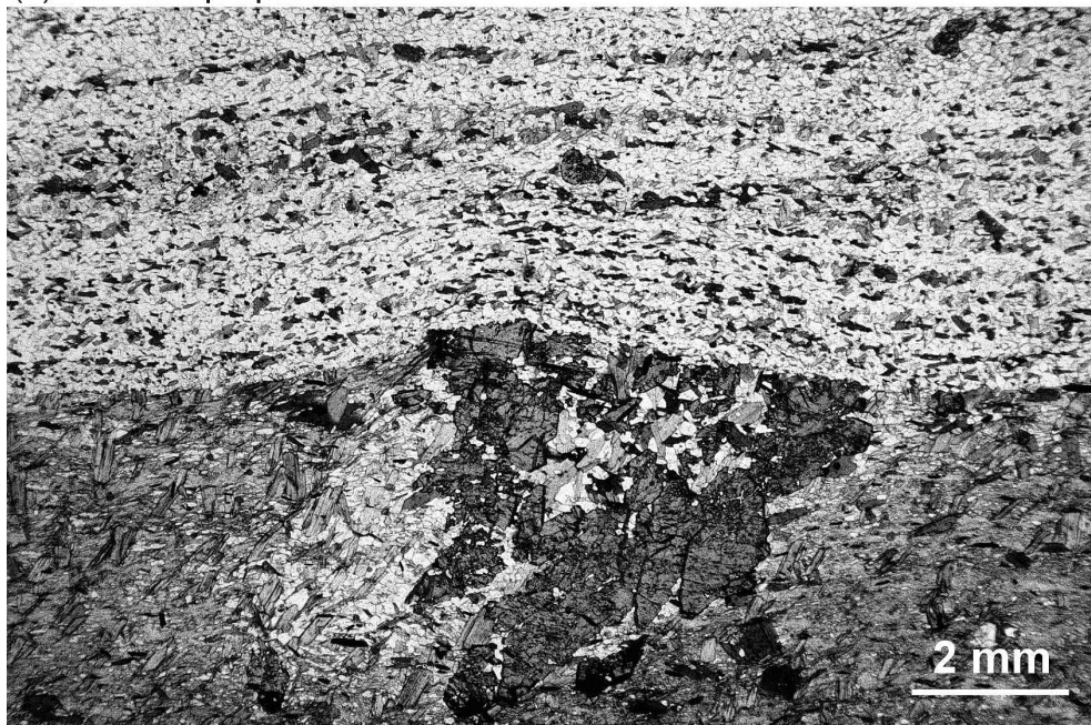
FIG. 1. Pair of transmitted plane-polarized light photomicrographs of thin sections cut orthogonally from a single oriented rock sample according to the grain-shape fabric as indicated. The sections are from a staurolite-garnet schist collected from the central HSZ (Perry Mountain Formation, Swift River, north of Coos Canyon, Byron, Maine). The strong blade-shape of micas is made apparent by comparing (a) and (b). Both views show the matrix fabric apparently flattened around the staurolite porphyroblast at bottom center, and both views show the staurolite to have inclusion trails that are not parallel to matrix foliation.
